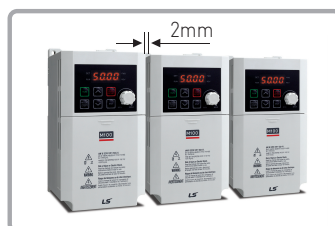
Side-by-side Installation (2mm between drives)
